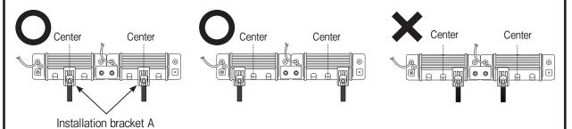
■ When installing and using "RF18" unit, make sure to install 2 Installation brackets A (Item ②) at 2 positions on each lamp.
