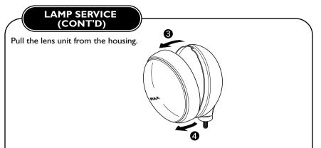
If the bulb is hot from use let it cool before touching or removing it from the lamp. To remove the main bulb (H4) unplug the socket from the back of the bulb. Release the wire retainer and pull the bulb out of the lamp. Remember to only touch the bulb by the metal base, do not touch the glass part of the bulb.
